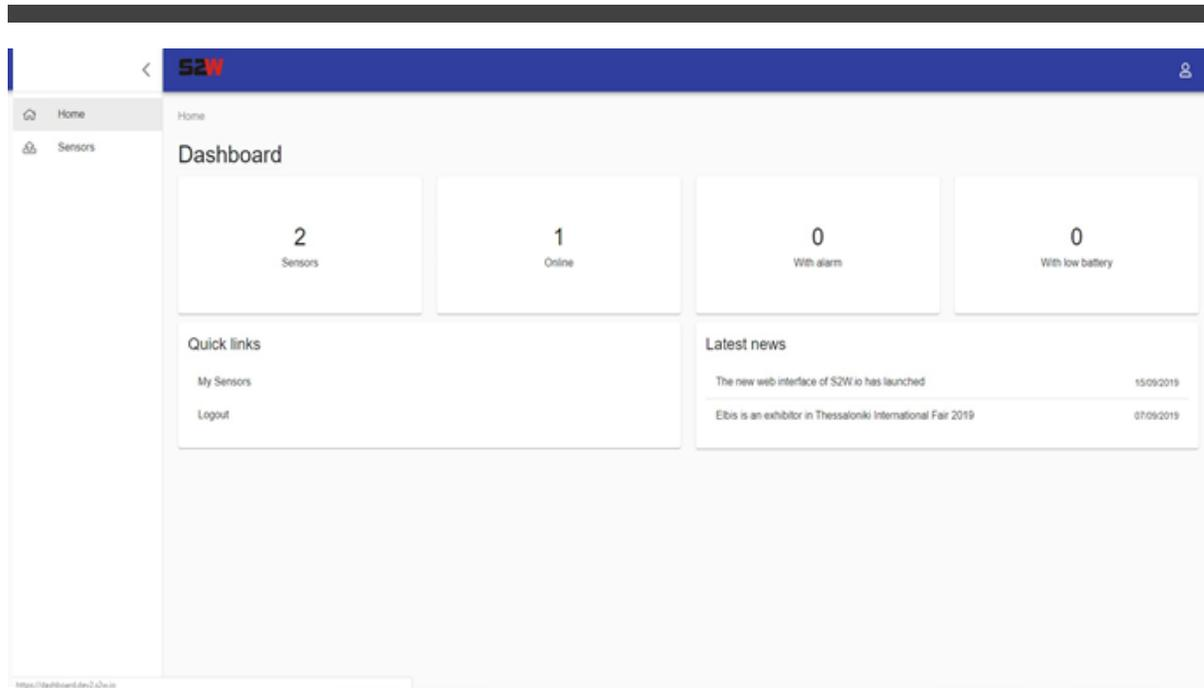
**Figure 8: Dashboard Homepage.** In this page you can view all your sensors, connectivity status, battery status and temperature alarms.
