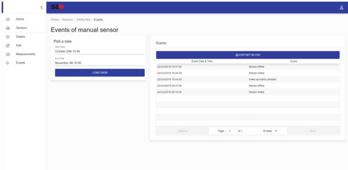
**Figure 14: Sensor’s Events page.** At this page the user can view the events history of the sensor. By picking up the dates he wants, events like connectivity status or "wake up button pressed" will appear.
