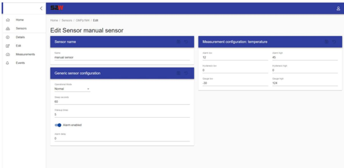
**Figure 12: Edit Sensor page.** By clicking on the **Edit** button, you can make a number of configurations, like sensor name, time settings (sleep seconds, wakeup times) and measurement configuration (high alarm, low alarm, hysteresis, gauge limits).
