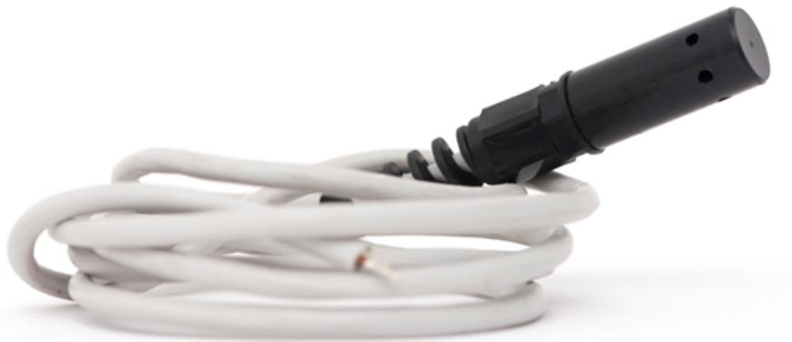
The **Sen-Humi** sensor probe is based on SHT21 digital temperature and humidity chip. It consists of **ABS cover** and **1 meter cable** with four (4) internal wires. Provides 8-bit to 12-Bit% RH relative humidity and 12-bit to 14-bit Celsius temperature measurements. The **Sen-Humi** communicates over a **I<sup>2</sup>C interface** that requires two (2) data lines for communication with a central microprocessor. In addition, the **Sen-Humi** is fully calibrated.
