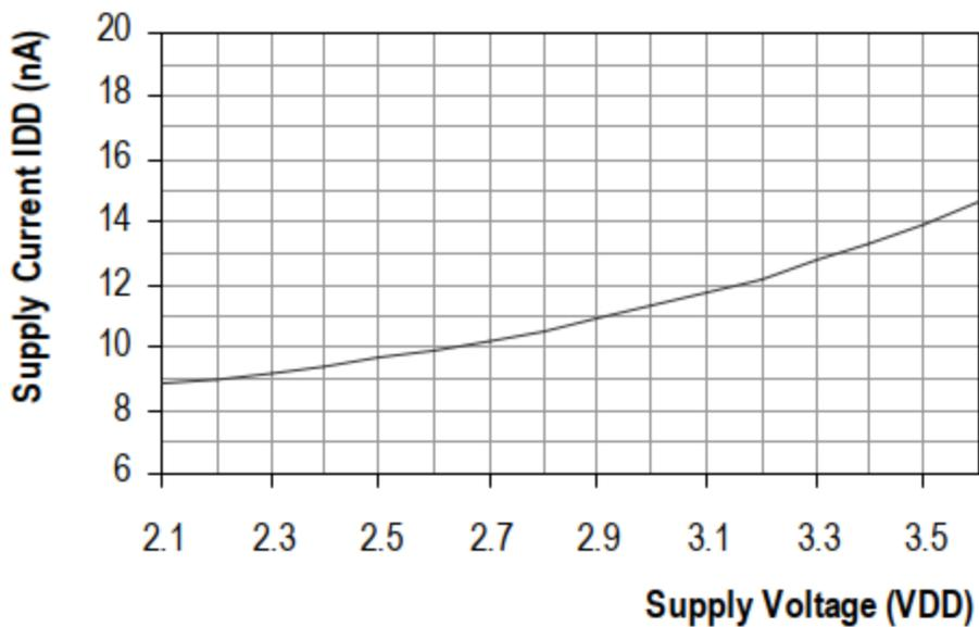
**Figure 7** Typical dependency of supply current (sleep mode) versus supply voltage at 25°C. Please note that deviations may be up to  $\pm 50\%$  of displayed value. Values at 60°C scale with a factor of about 15 (compare Table 1).
