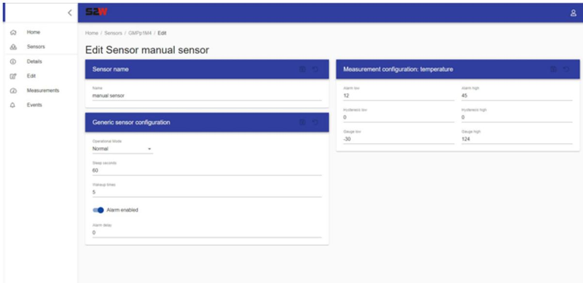
**Figure 12: Edit Sensor page.** By clicking on Edit, you can make a number of configurations, like sensor name, time settings (sleep seconds, wakeup times) and measurement configuration (high alarm, low alarm, hysteresis, gauge limits).
