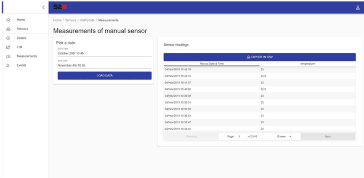
**Figure 13: Sensor’s Measurements page.** At this page, user can handle all the data measurements history and can export them at an excel or pdf file for analysis and back up.
