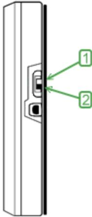
**Figure 5** (Power Switch 1:Off, 2:On)
