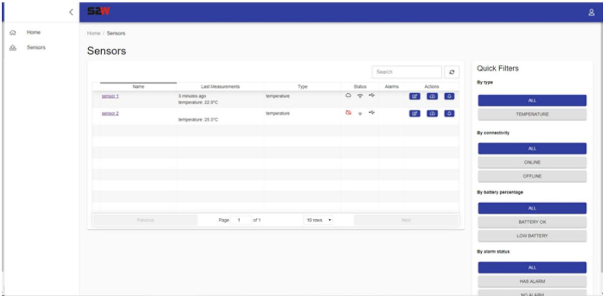
**Figure 9: List of Sensors page.** If you choose **Sensors**, you will be transferred to the main sensor page. Here, the user can view all the sensors with more than the basic information, e.g. when last measurement of temperature was taken, alarm limits and connectivity. At the right side of the page, you can view the quick filters that help you to categorize the sensors by different status..
