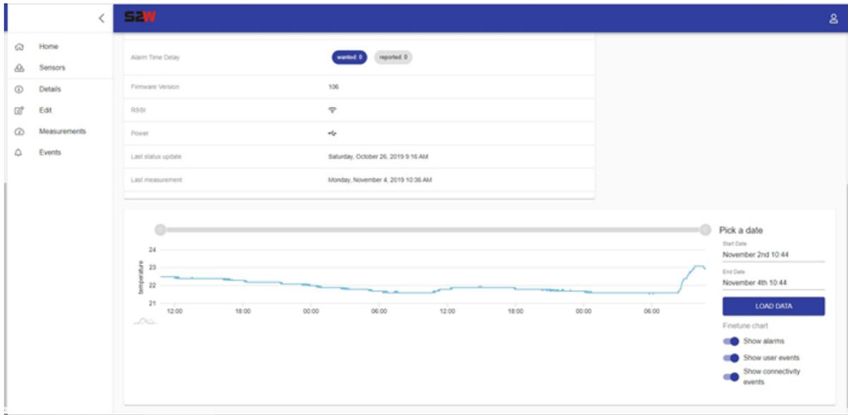
**Figure 11: Sensor Details page.** Click on the sensor you want, to see all the details of the sensor (sensor type, measurement time, operational mode, alarm delay etc). At the right side of the page there is a temperature gauge where you can see the last measurement. Also, at the bottom of the page there is a temperature measurement chart. Pick a date and view the waveform chart.
